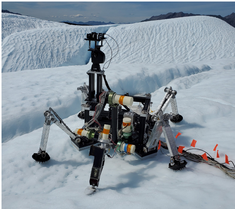
▲ A Europa Lander mockup excavates ice on Matanuska Glacier in Alaska to simulate autonomous subsurface sample collection where potential biosignatures may be protected from Jupiter's radiation. Stereo cameras atop the lander allow it to perceive its environment, and cables coming out of the base provide offboard power and computation.
