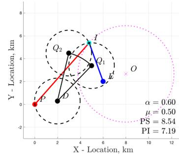
Fig. 4. The directed energy defense scenario where the bearing from the pursuer to the defender is 40 deg starboard. The speed ratio between the evader to the pursuer is  $\mu = 0.50$  and the speed ratio between the defender and the pursuer is  $\alpha = 0.60$ .
