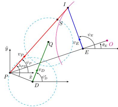
Fig. 1. The directed energy defense scenario wherein the maximum possible exposure time is less than the time-to-go.
