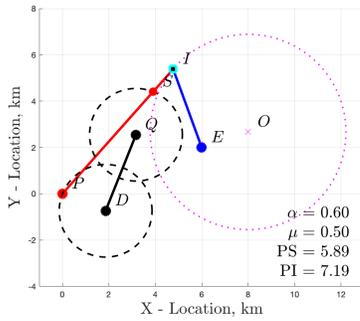
Fig. 3. The directed energy defense scenario where the bearing from the pursuer to the defender is 70 deg starboard. The speed ratio between the evader to the pursuer is  $\mu = 0.50$  and the speed ratio between the defender and the pursuer is  $\alpha = 0.60$ .
