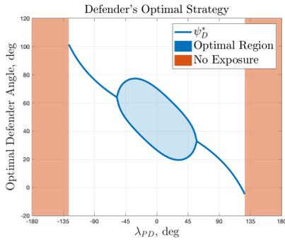
Fig. 6. The defender's heading ( $\psi_D$ ) as a function of the line of sight angle  $\lambda_{PD}$  as described in (47). The case presented is that of the examples where  $E = (6, 2)$ ,  $\alpha = 0.6$ , and  $\mu = 0.50$ .
