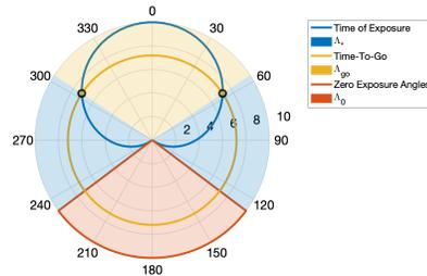
Fig. 5. The exposure time as a function of the line of sight angle  $\lambda_{PD}$  is depicted in this polar plot when  $E = (6, 2)$ ,  $\alpha = 0.6$ , and  $\mu = 0.50$ . This polar plot is a graphical representation of (44)
